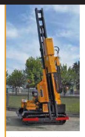
Hydraulic system to adjust the column for vertical position.
