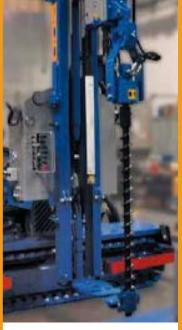
PILE DRIVER WITH HYDRAULIC AUGER
