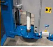
DOWN THE HOLE HAMMER IN "STAND-BY" POSITION
