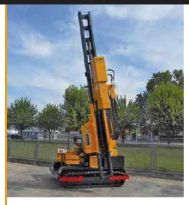
**CORRECTION OF VERTICALITY**Hydraulic system to adjust the column for vertical position.
